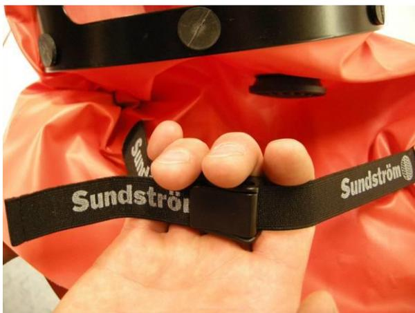
In emergency situations, the neck strap can be released without releasing the buckle:
