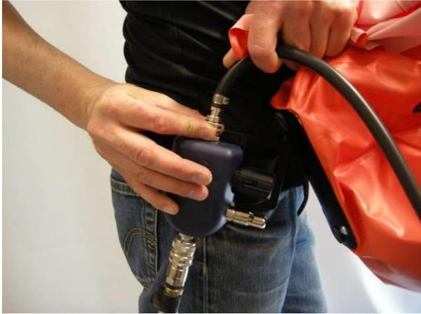
Releasing the compressed air tube / breathing hose
