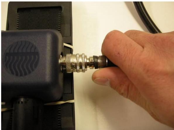
On every occasion before the hood is used, check that the air flow - measured in the hood - is at least 150 l/min.
