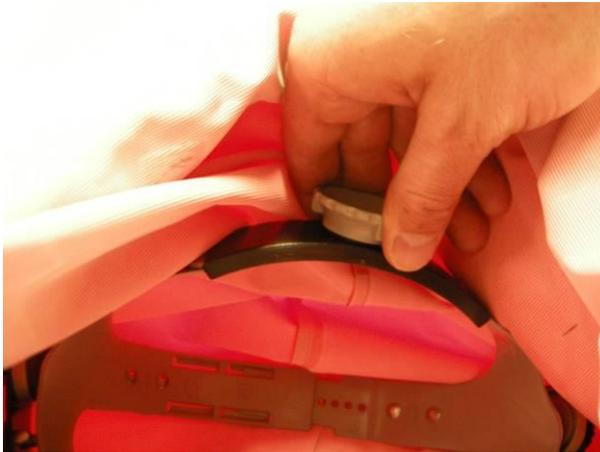
The width and height can be adjusted with the head harness in place in the hood.
