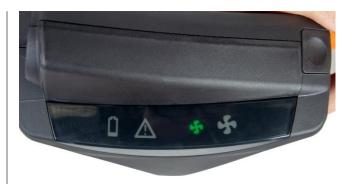
**6.3** After the internal test, all symbols will be extinguished except the small green fan symbol. This indicates normal operating status with a flow of at least 175 l / min.
