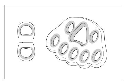
• Check the condition of the attachment holes (marks, deformation, cracks, corrosion...).
