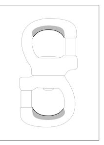
· Check for wear caused by rope movement, or by contact with anchors (depth of marks: retire your SWIVEL if it shows any wear greater than one mm deep. Check for the presence of any sharp edges...).
