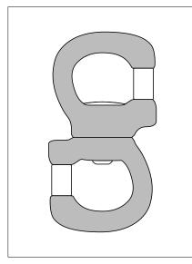
• Check the condition of the frame (marks, wear, cracks, deformation, corrosion...).
