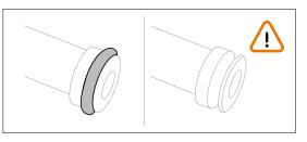
• Verify the presence and the condition of the o-ring on the screw heads.
