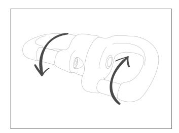
• Check the bearing for smoothness of rotation, in both directions. Make sure there is no excessive play between the two parts of the frame.
