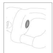
• Check the condition of the axle rivet (marks, wear, cracks, deformation, corrosion...).
