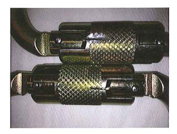
The attached picture shows two of the same type of carabiner (P/N 10089207). The bottom gate is normal. The top one has had some of the knurling ground off in order to show the full width of the machined slot.
