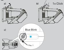
In boost mode, the lamp lights up with the maximum brightness for 10 sec. The boost mode can be activated only in the switched on state (but not in strobe mode).
