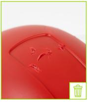
External shell with impact deformation
