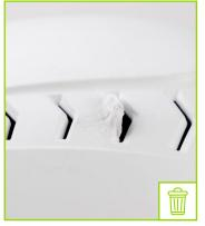
Shell with deformed ventilation hole
