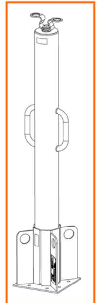
Conform to EN 795 classe A-1 : Anchorage point
