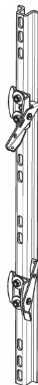
Fig. 11 Example of steel fall arrest rail with movable end stops Model A and Model B
