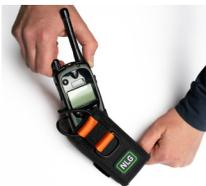
Insert the radio into the holster and position the two bungee cords to pass over the top controls of the radio.
