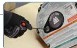
Remove the two shoulder screws on the drum through the side plate cover.
