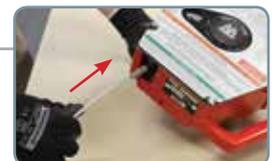
Insert new lifeline into the unit, install shoulder screws and ensure it has engaged.
